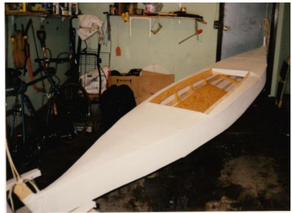
Wrapped up, ready for water proofing
